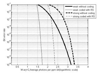
Fig.1. Comparison of non-coded BPPM in weak turbulence of 0.3 scintillation index with Reed Solomon (255,207) and in strong turbulence of 1.0 scintillation index.
