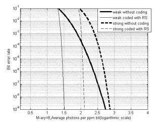
Fig. 2. Comparison of non-coded 8-PPM in weak turbulence of 0.3 scintillation index with Reed Solomon (255,207) and in strong turbulence of 1.0 scintillation index.
